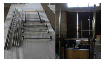
Step 11. Connect the stainless steel cross frame and the longitudinal tube, then place it on the main stand riser and tighten the screws.
