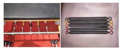
Step 8. Locate the tension cord and install it on the car through the pulley.
