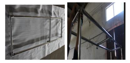
Step 12. Attach the spring, handle and other accessories to the main frame as shown below. Springs for Full Trapeze Table:four in red (0.5 resistance) and four in black (2 resistance).
