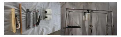
Step 13. When installing the flat bed, take the limit post down, place the flat bed on the main frame, and use the Phillips screw to hold the car against the sway.
